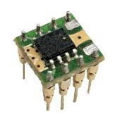
AS394-HYB (AS194-HYB) is a DIP-8 module which contains matched monolithic NPN transistor pair AS194/394DE (with an order of magnitude improvement in matching over conventional transistor pair ) with improved heatsink possibility and place for mounting SMT thermosensor (2010 size). Electrical parameters - according to datasheet of AS194DE/AS394DE ( <a href="http://www.alfarzpp.lv/eng/sc/AS394CH.pdf">http://www.alfarzpp.lv/eng/sc/AS394CH.pdf</a> )
